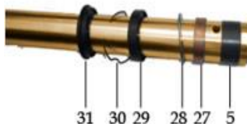
(31) SCRAPER (30) CLIP (29) SEAL (28) WASHER (27) PISTON METAL (5) SLIDE METAL
